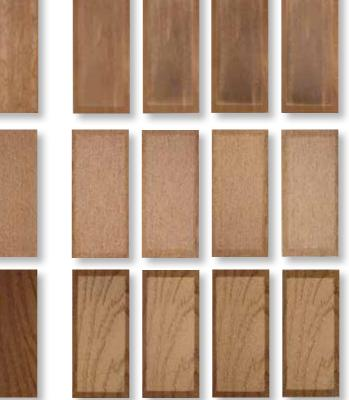
Wood + Polymer (WPC) clearly visible change in color (bleaching), brittle and cracked surface, several white particles individually visible
